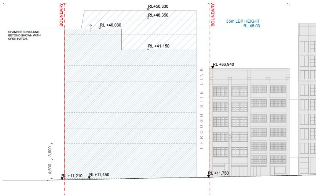
Figure 15. Proposed building envelope – Reservoir Street elevation
